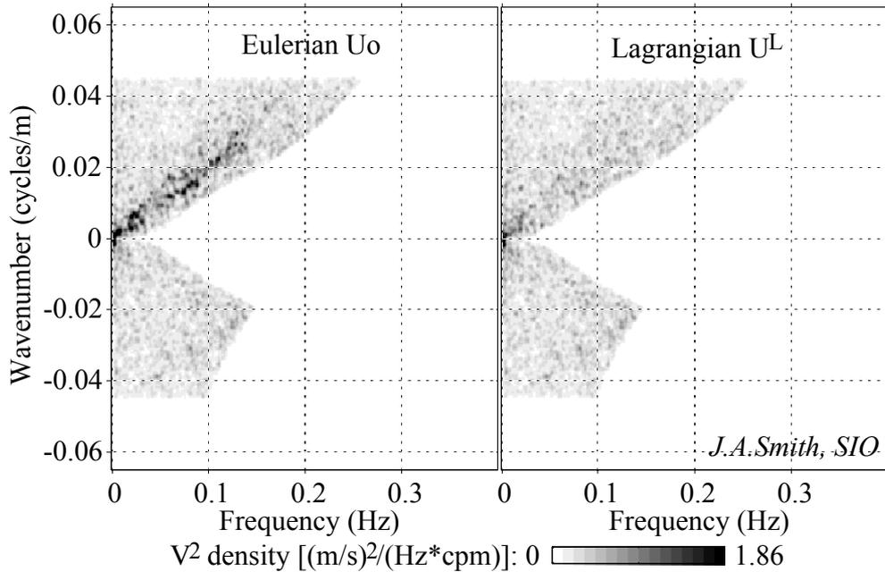
Fig. 5: Wavenumber-frequency spectra for (left) the Eulerian velocity field and (right) the Lagrangian velocity field formed by adding the Eulerian and Stokes drift estimates. The greyscale is linear in variance density, not logarithmic as in Fig. 3. The reduction in variance along the 5 m/s line in the Lagrangian field is dramatic. The remaining variance on the right ( $U^L$ ) is close to the spectral noise floor.
