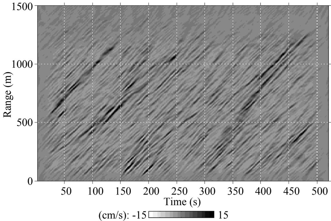
*Fig. 4: Time-range plot of the radial Stokes drift for the same segment as in the previous figures (time-means at each range are removed). Note the predominance of slashes at an angle corresponding to roughly 5 m/s propagation along the beam..*
