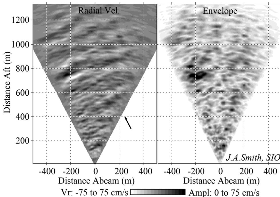
*Fig. 1: Example LRPADS image of the surface wave field, showing radial (roughly horizontal) surface orbital velocity component (left panel). The right panel shows the complex amplitude (envelope) of the waves. The black arrow indicates the wind direction and magnitude (near 10 m/s). The waves are propagating roughly downwind.*
