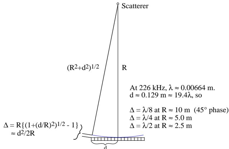
Fig. 2 The need for focus. In practice, the 5 m cutoff ( $90^\circ$  phase criterion) appears the most appropriate; beyond this the images produced with and without focusing adjustments are hard to distinguish.
