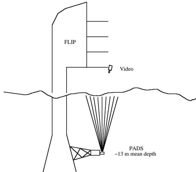
Fig. 1: Schematic of the deployment on FLIP. The experimental site was some 200 West of San Diego, in 4 km water depth.
