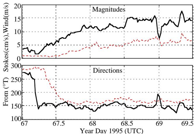
Figure 19.3 Wind (solid curve) and Stokes' drift (dashed curve) over the focus time segment of MBLEx leg 1. Note the delay between the onset of wind and development of Stokes' drift. Just prior to this segment, the wind was from the NW, and swell continued to come from that direction, explaining the slow reversal in Stokes' drift direction. Similar data were gathered for the SWAPP experiment.
