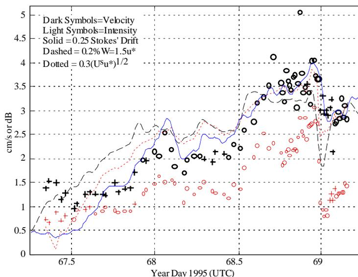
Figure 19.7 RMS radial velocity (dark symbols) and intensity (light symbols) associated with the features, versus time. Each symbol represents a half-hour average; crosses represent dubious estimates, circles more reliable ones. For scaling and comparison,  $0.25U^S$  (solid line),  $0.002W$  (dashed line), and  $0.023(U^S W)^{1/2}$  (dotted line) are also shown.
