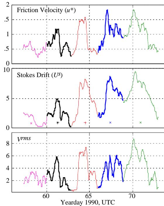
Figure 19.4 Wind, waves, and rms surface velocity during SWAPP. The first segment has weak variable winds; the last segment contains several directional shifts; the second-to-last segment has little variation in the ratio  $U/u^*$ . Thus, only the second and third segments are suitable for testing the relationship between the three parameters.
