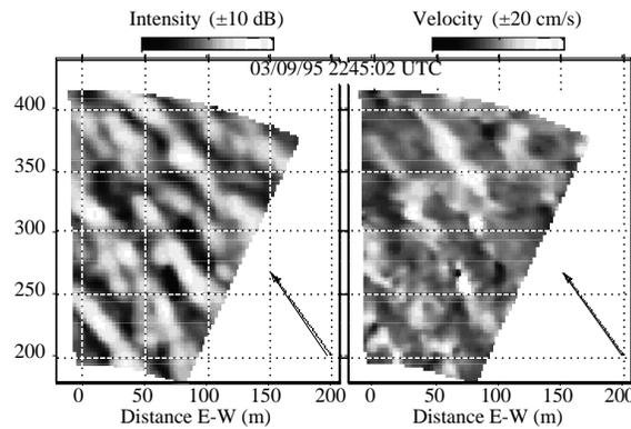
Figure 19.1 Example frame of PADS data: (left panel) Acoustic backscatter intensity; (right) Radial velocity. The arrows indicate wind speed and direction; the arrow shown represents a 15 m/s wind. North is up. The data are smoothed to 3 minute averages, modified to “track” the mean flow across the area.
