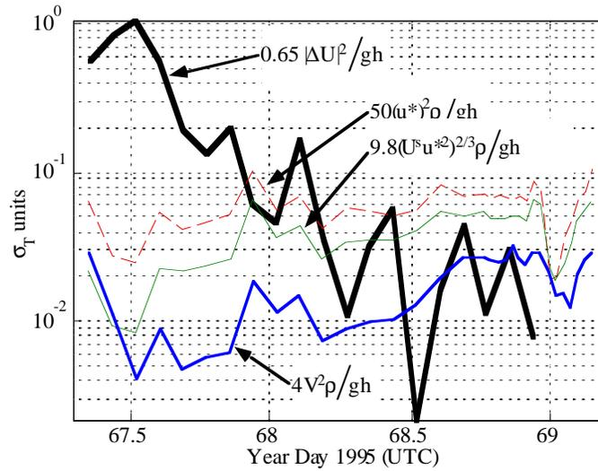
Figure 19.6 Mixing strength, parameterized by the density jump required to stop mixing, for (1) the bulk Richardson (or PRT) mechanism (thick line); (2) Langmuir circulation, as estimated directly from the rms velocity scale  $V$  (medium line); and (3) LC mixing estimated from  $U^s$  and  $v_t$  via comparison with numerical model results, for developing waves (thin solid line) and for fully developed waves (thin dashed line).
