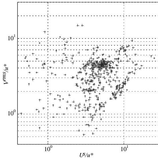
Figure 19.9 All data points from SWAPP and MBLEX-1, plotted without regard to event or whether LC features were identified. No correlation is seen, and it appears that almost an order of magnitude uncertainty in  $V^{rms}$  must be tolerated.
