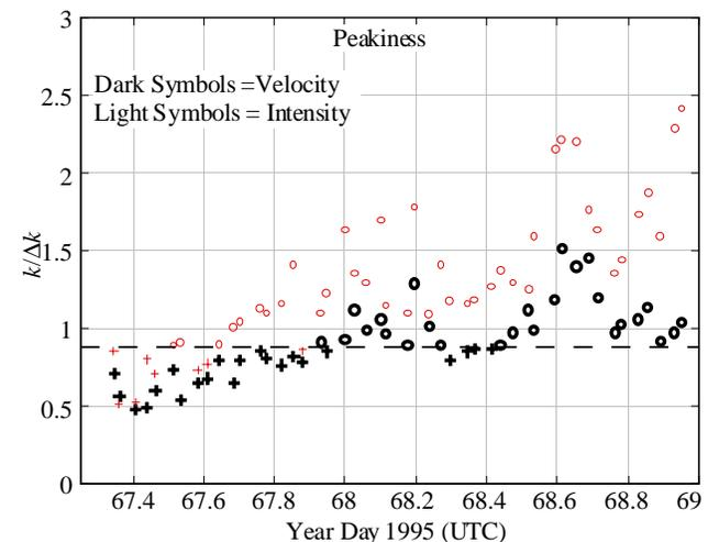
**Figure 10.** Peakiness index for intensity (light symbols) and radial velocity (dark symbols). The peakiness is also used as an indicator of quality: here, and in the related Figures, crosses represent cases where the peakiness falls below  $7/8$  (dashed line).
