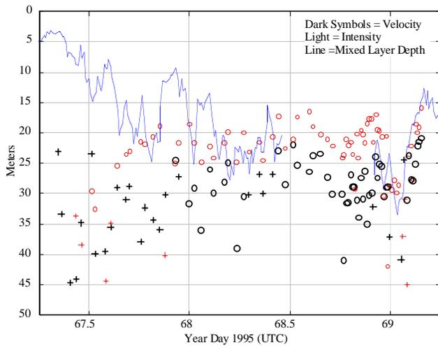
**Figure 8.** Half the feature spacing versus time (symbols), and mixed layer depth (solid line). Crosses represent dubious data. Note the velocity feature spacing (darker circles) generally lies below that of intensity (light circles). This relation indicates that the rolls are approximately as deep as they are wide.
