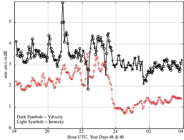
**Figure 12.** The rms radial velocity (dark symbols) and intensity (light symbols) over the close-up segment. The vacillations are clearest between 2130 and 2330, year day 68. The velocity variations are exactly opposite to those of intensity: maximum intensity feature strength corresponds to minimum rms velocity.
