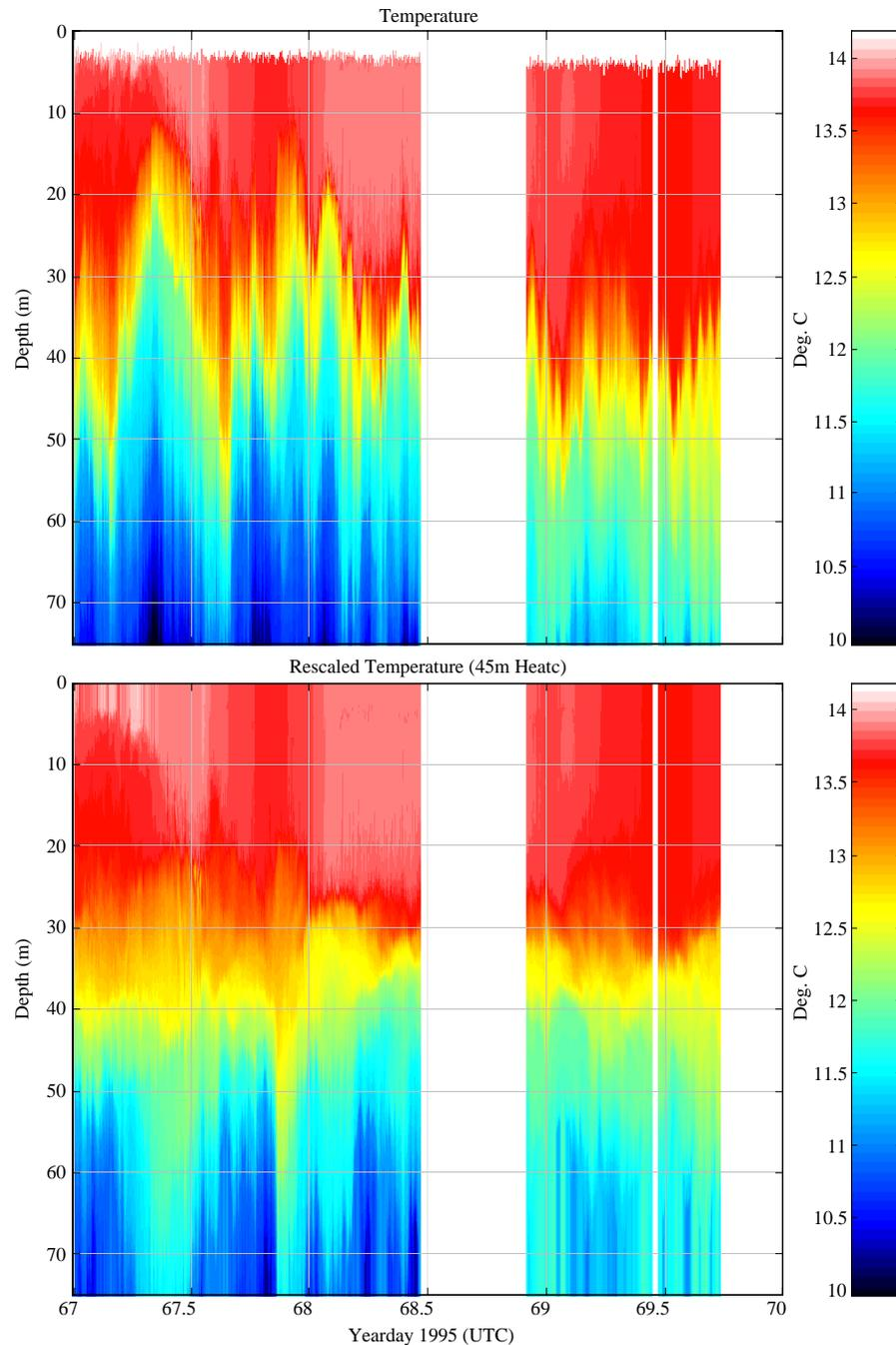
**Plate 1.** (top) Temperature profile time series and (bottom) stretched profiles. Linear stretching of the vertical coordinate is adjusted to make the (stretched) heat content from 0 to 45 m depth constant. This should reduce the effect of low-mode reversible processes (e.g., internal waves or quasi-geostrophic activity).
