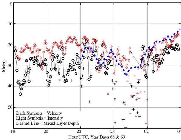
**Figure 13.** Half the spacing (connected symbols) and mixed layer depth (dashed line). During the vacillations (2130 to 2330), the spacing of features in both intensity and radial velocity oscillates together, with minimum spacing coinciding with maximum intensities, minimum velocities (compare with Figure 12). After the wind drops, just before 0000 day 69, the mixed layer shoals. Plate 1 indicates this is partly accounted for by low-mode "vertical stretching."
