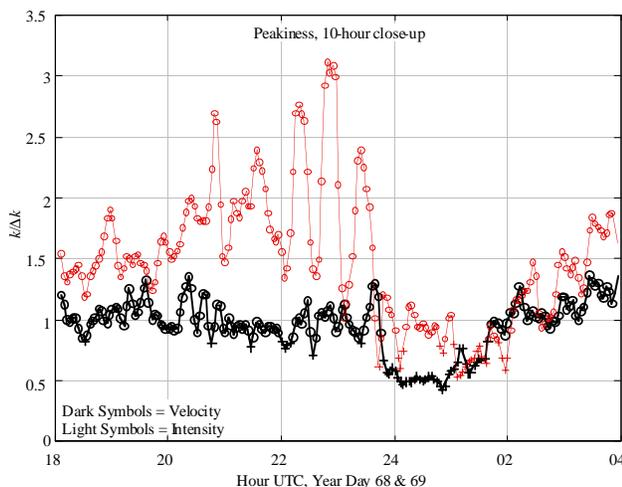
**Figure 11.** Peakiness index over the 10-hour close-up period. Vacillations are prominent in the intensity peakiness (lighter symbols) but absent in the velocity peakiness (darker symbols). The wind shifts at 2330, causing the features to fade; they rebuild slowly as the wind shifts back and picks up to 15 m/s again.
