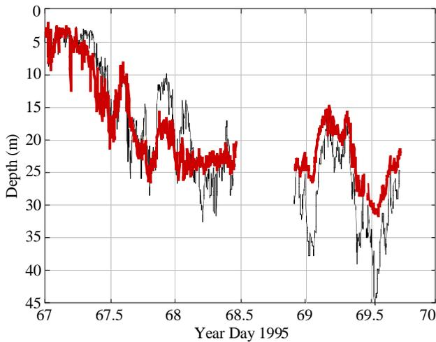
**Figure 15.** The mixed layer depth over the whole focus period, evaluated as the depth at which the temperature falls to  $0.05^\circ\text{C}$  below the value nearest the surface. Thin line shows “raw” MLD; thick line, MLD from the vertically scaled temperatures (as in Plate 1, bottom).
