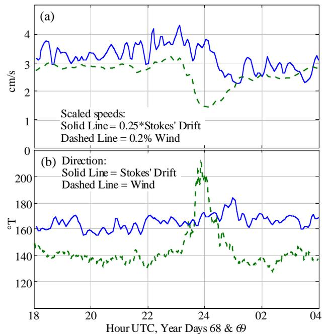
**Figure 14.** (a) Scaled wind speed  $W$  (dashed line) and Stokes' drift  $U^s$  (solid line) and (b) their directions. No "vacillations" in wind speed or direction are seen. Careful comparison of the noisier Stokes' drift estimate shows that the variability is not correlated with the vacillations in the intensity and radial velocity features.
