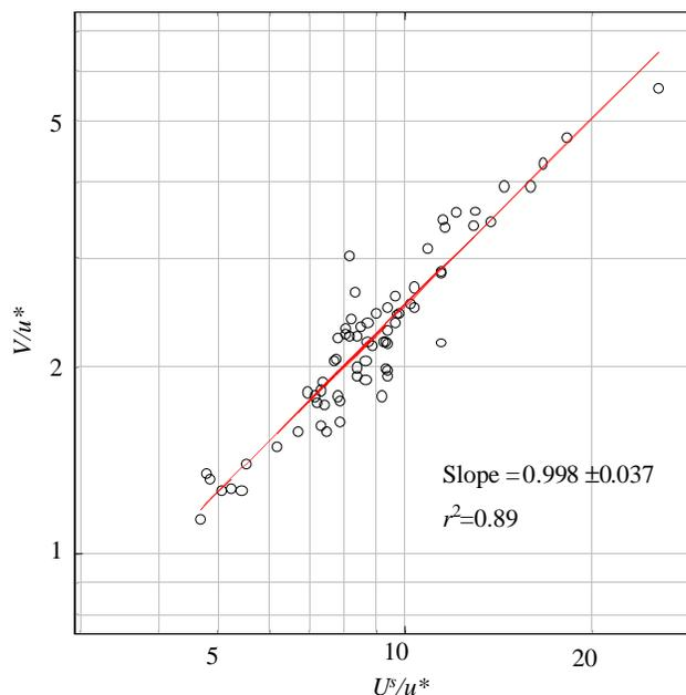
**Figure 7.** Scaling of the rms measured radial surface velocity takes the general form  $V \sim u^*(U^s/u^*)^n$ . The value of  $n$  is sought as the slope of  $(V/u^*)$  versus  $(U^s/u^*)$  on a log-log plot. This Figure indicates a well-determined value for  $n$  very near 1.0; i.e.,  $V \sim U^s$ , with no dependence on  $u^*$  once Langmuir circulation is well formed. Values before year day 67.66, when there were no signs of Langmuir circulation, were excluded from this plot.
