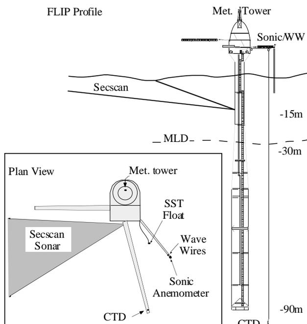
**Figure 2.** Plan and profile views of *Flip*, MBLEX leg 1, showing various instrument locations. The phased array and SW sonars were mounted on an active heading compensation system, maintaining bearing to within  $0.1^\circ$  rms.
