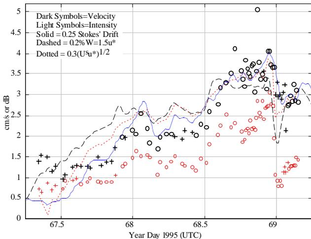
**Figure 6.** RMS radial velocity (dark symbols) and intensity (light symbols) associated with the features, versus time. Each symbol represents a half-hour average; crosses represent dubious estimates, circles more reliable ones. For scaling and comparison,  $0.25U^s$  (solid line),  $0.002W$  (dashed line), and  $0.023(U^s W)^{1/2}$  (dotted line) are also shown.
