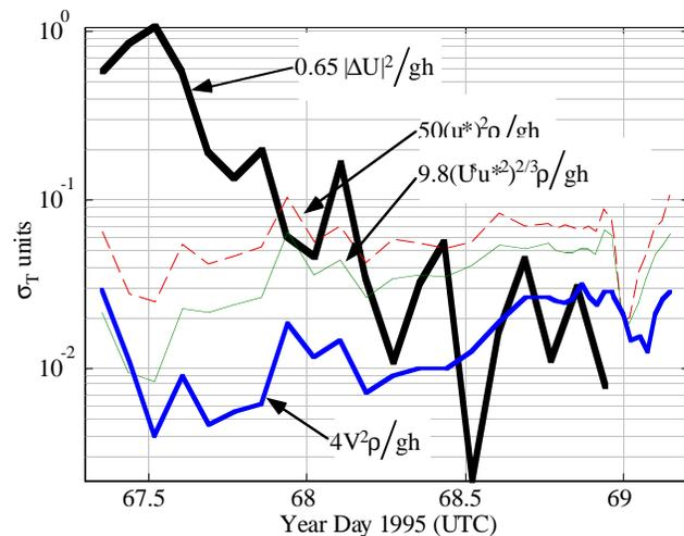
**Figure 16.** Mixing strength, parameterized by the density jump required to stop mixing, for (1) the bulk Richardson (or PRT) mechanism (thick line); (2) Langmuir circulation, as estimated directly from the rms velocity scale  $V$  (medium line); and (3) LC mixing estimated from  $U^s$  and  $v_t$  via comparison with numerical model results, for developing waves (thin solid line) and for fully developed waves (thin dashed line).
