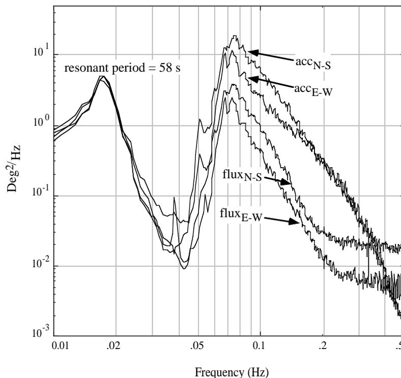
Fig. 2. North-South and East-West (acc) accelerometer and (flux) fluxgate equivalent spectra As enforced by calibration, the spectra match at the tilt resonant period of 58 seconds, but at higher frequencies, the effect of waves, which accelerate *FLIP*, can clearly be seen.
