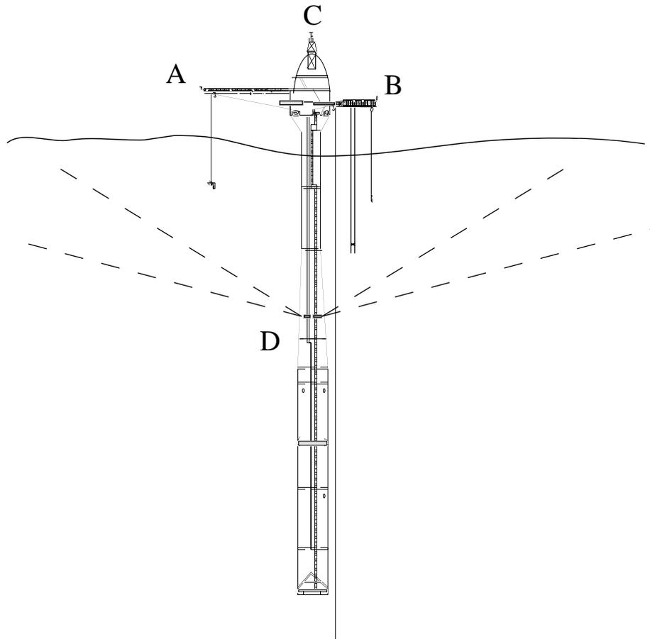
Fig. 1. Schematic view of R/P *FLIP* during SWAPP Instruments deployed included: (A,B) high frequency sonic anemometers, (C) vector-averaging wind recorder, and (D) surface scanning Doppler sonars.
