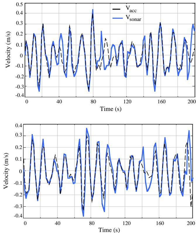
Fig. 5. Time-series of (grey) accelerometer-derived velocity at the sonar depth, via *FLIP* motion model, and (black) the sonar range-mean velocity for two time periods: (top) March 11, 1990, 20:29, and (bottom) March 13, 1990, 1:47.
