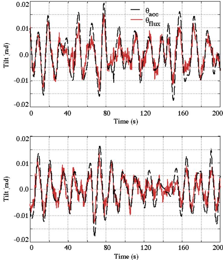
Fig. 4. Time-series of (grey) accelerometer-derived tilt, via *FLIP* motion model, and (black) fluxgate measured tilt, for two time periods: (top) March 11, 1990, 20:29, and (bottom) March 13, 1990, 1:47.
