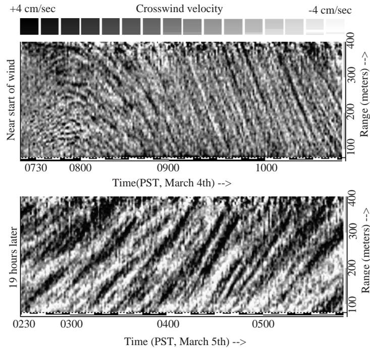
Figure 4. Two samples of sonar velocity data from SWAPP. The first sample is near the beginning of a wind event. The wind increased suddenly at about 7:30; just after that, small "ripples" are apparent, especially near 150m range. After that, there is rapid evolution toward larger scales; also the mean flow increases, creating the diagonal stripes seen over the second half of this sample. The second sample is some 19 hours later, and shows "fully developed" Langmuir circulation.
