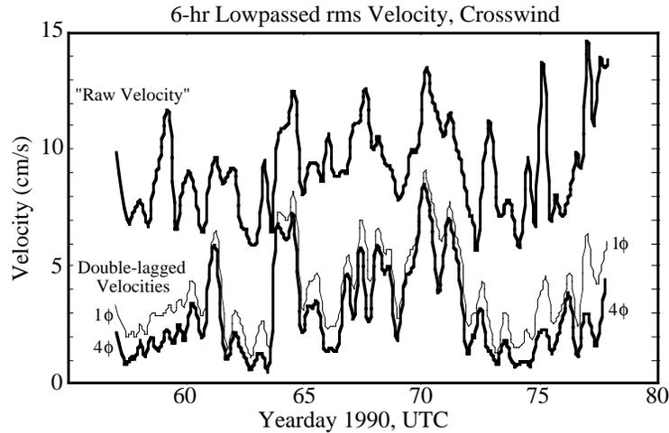
Fig. 8. The noise reduction effected by the "Double-lagged covariance" processing (see text).
