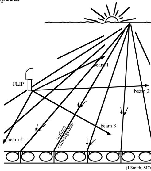
Fig. 3. Schematic view of Langmuir circulation and the 4 sonar beams extending from FLIP.
