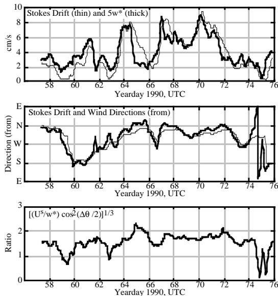
Fig. 11. Surface Stokes' drift ( $U^S$ ) and water friction velocity ( $w^*$ ) over the course of SWAPP, smoothed with a 6 hr running mean. (a) Magnitude; (b) Direction; (c) Ratio of scaling factor to  $w^*$  (see text).
