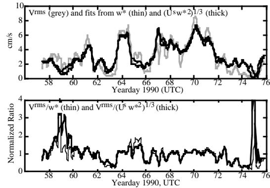
Fig. 12. Comparisons between  $V_{rms}$  (grey) and fits from just  $w^*$  (thin lines) versus the theoretical scaling  $(U^S w^{*2})^{1/3}$  (thick lines). (a)  $V_{rms}$  and the scaling fits; (b) The ratio of  $V_{rms}$  to the scaling fits. Ignoring times when all three are small (days 59, 63, and 75), the only significant difference occurs on day 65, when the Stokes' drift remains anomalously high.
