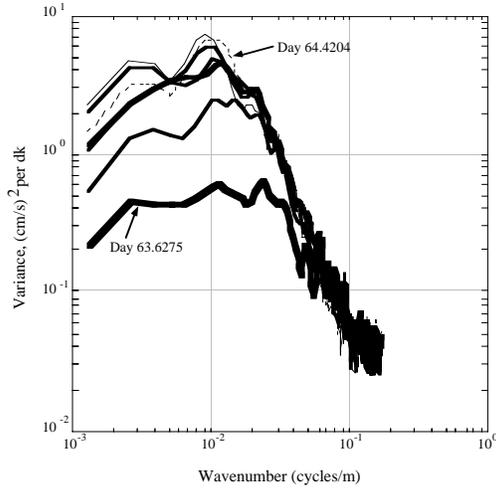
Fig. 6. Time-lagged cospectra of velocity from the Doppler sonar data. Six hour averages, 3 hour intervals displayed.
